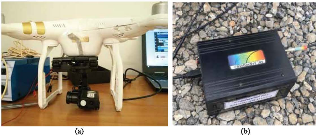
Figure 3: (a) Modified infrared camera setup with 3 axis brushless gimbal on DJI P3 Professional, (b) Spectrometer (Black Comet C-200 TEC ranging from 200-1100nm)
