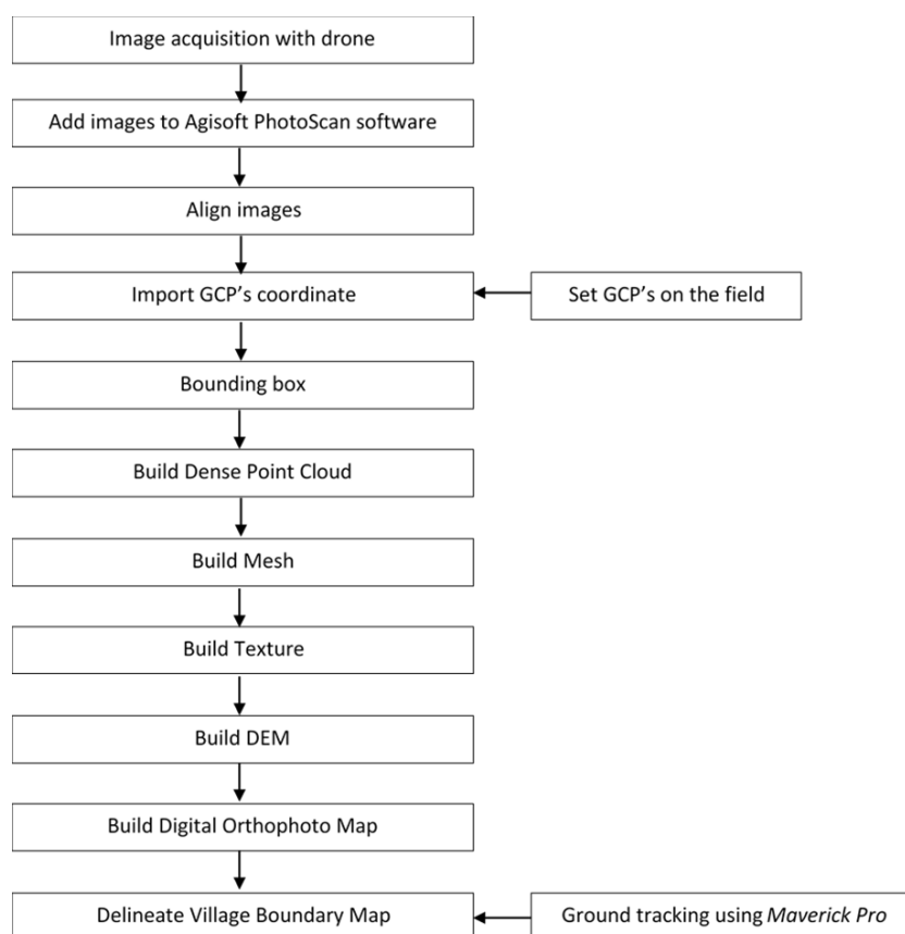
Figure 3: Workflow to produce the orthomosaic under Agisoft PhotoScan software environment
