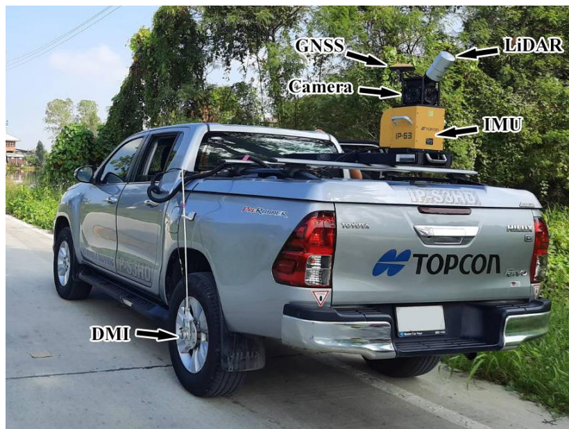
Figure 2: MMS-IP-S3 mounted on a vehicle
