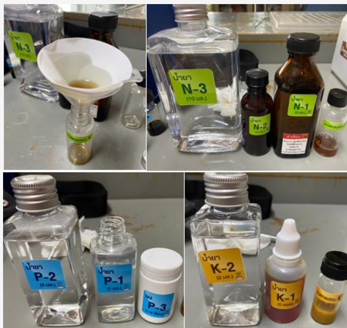
Figure 7: Field soil inspection kit (LDD test kit)
