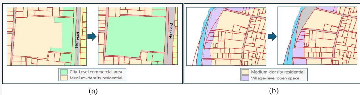
Figure 13: Example of geometric harmonisation; (a) accessibility aspect consideration; (b) rigidity aspect consideration
