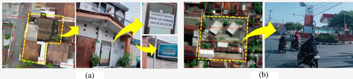
Figure 11: Specific phenomena of spatial utilisation in cadastral land parcel-based evaluation; (a) example of one cadastral land parcel with multi-land utilisation; (b) one-land utilisation with multi-cadastral land parcel
