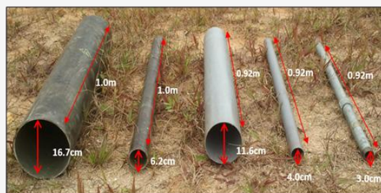
Figure 2: The length and diameter of the fiberglass pipes, PVC pipe diameters, and metal pipe
