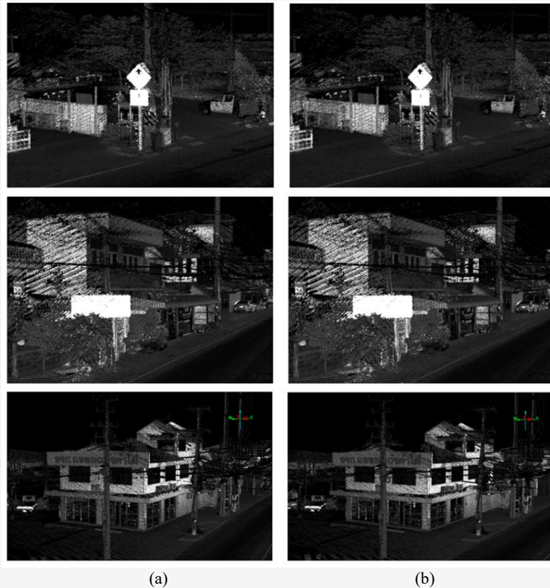
Figure 21: Georeferenced point cloud of the experiment in open-sky condition using different antenna configurations (a) single antenna (b) dual antenna
