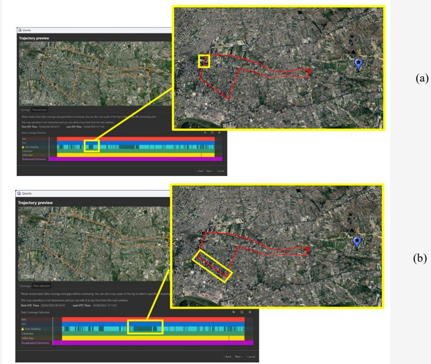
Figure 11: The time interval of prolonged Dual GNSS-estimated heading data outage in urban area: (a) GPS time 120837 to 121207 seconds and (b) GPS time 123130 to 124592 seconds
