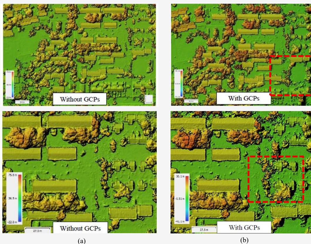
Figure 9: Comparison of DSM results: (a) with GCPs, and (b) without GCPs
