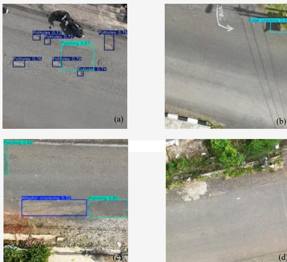
Figure 4: Pavement distress detection results using the YOLO deep learning model from UAV orthophoto imagery: (a) True positive (b) False positive (c) False negative (d) True negative
