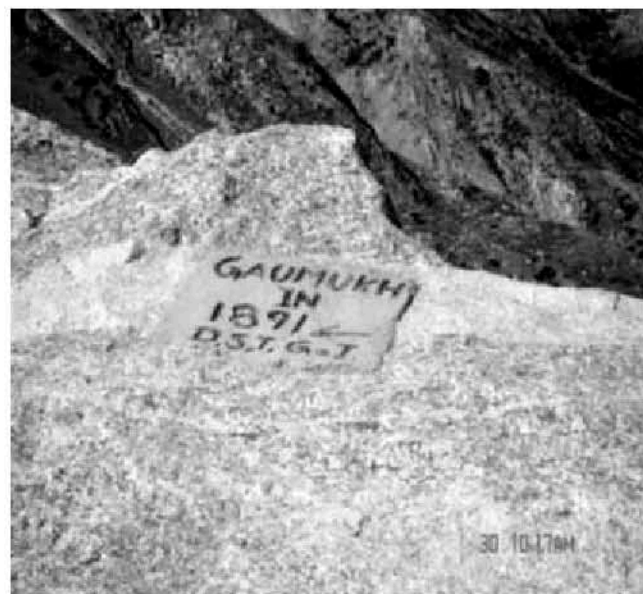
Figure 2: Cemented benchmark on the huge boulder set up by D.S.T. (GoI) in the field showing snout position for 1891.
