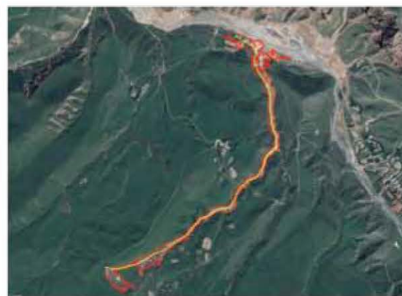
Figure 4: Landslide polygon (red) and its length line (yellow) derived automatically with QGIS plugin
