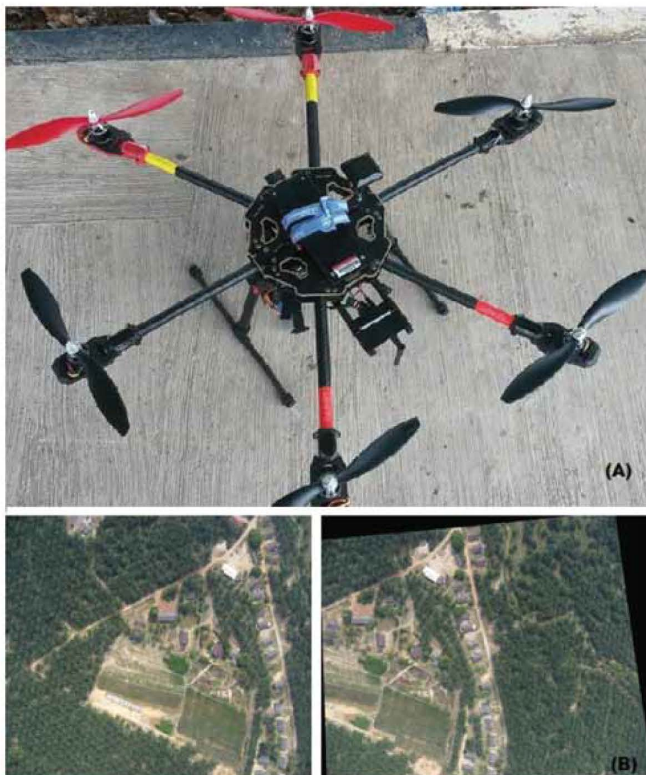
Figure 1: Multi-rotor UAV (a) assembled with a Canon - PowerShot SX-230 HS digital camera and all other accessories, fully prepared for data collection and ready for take-off. And (b) is the two adjacent UAV images used for testing the performance of RI-SIFT algorithm for keypoints extraction
